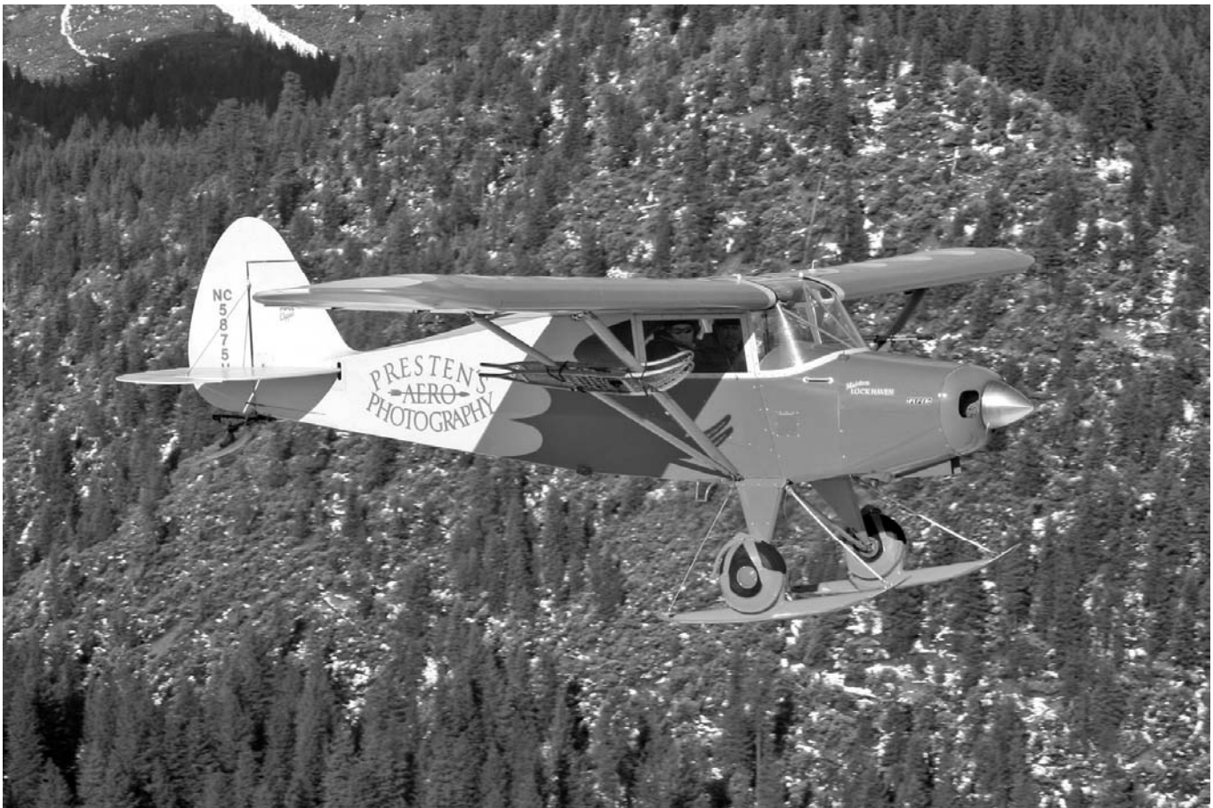
Above: Eric and Debbie Presten fly their 1949 Piper PA-16 Clipper over the town of Quincy, on a pair of 1948 Federal Aircraft Works skis. Unlike the traditional type of snow skis that require removing the wheels and brakes, these simply clamp-on, making for a quick conversion from pavement or field to
